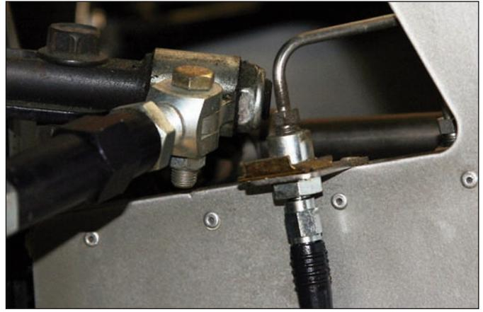
**Sequence 21:** Connect one end of the flexline to the previously installed caliper fitting. Route line along the same path as the OEM hose and connect the other end of the flexline to the fitting at the brake hard line. Secure line as necessary to prevent contact with moving suspension, brake, or wheel components. Bleed the system referring to the additional information in the data sheet as necessary for proper bleeding instructions.
