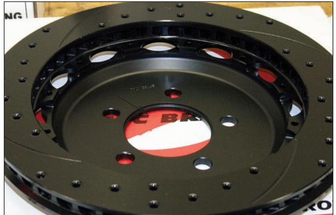
**Sequence 11:** The hat needs to be bolted to the rotor. Orient the rotor over the hat in the configuration shown above.
