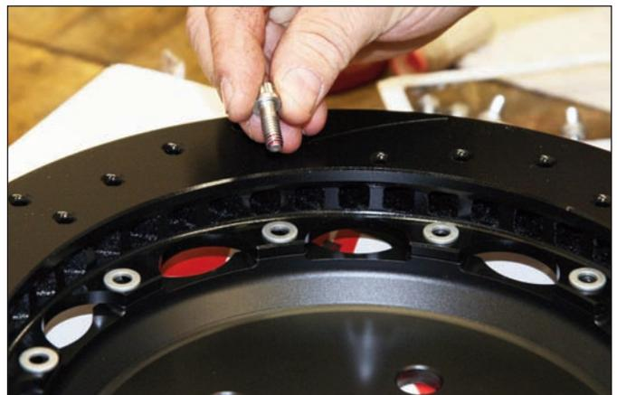
**Sequence 12:** Place one flat washer over each hole on the rotor mounting tabs. Coat the mounting bolts with red *Loctite*® 271 and slide through the washer and thread into the hat. Using an alternating sequence, torque bolts to 155 in-lbs.
