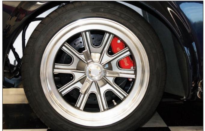
**Sequence 22:** Install the wheel and torque the lug nuts to manufacturer's specification. Rotate the wheel and check for any interference. Reinstall the replica knock-off's. Bed in the brake pads and rotor in a safe location before general use driving.
