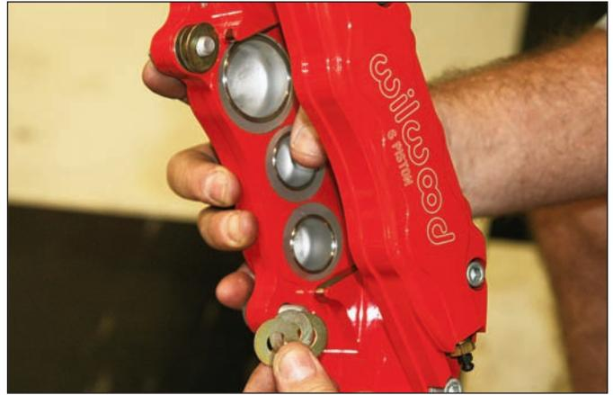
**Sequence 16:** Initially place three shim washers on each bolt between caliper mounting tab and the mounting ears on the bracket.
