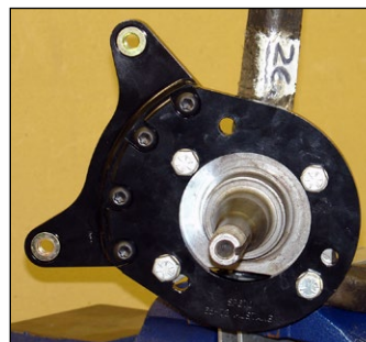
Photo 1 (4-Bolt Spindle Mounting)
