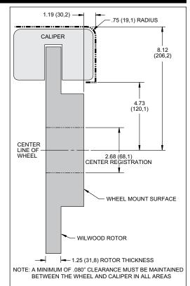
Figure 2. Wheel Clearance Diagram
