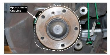
Photo 1, Dust Shield Modifications (Left Side Shown)
