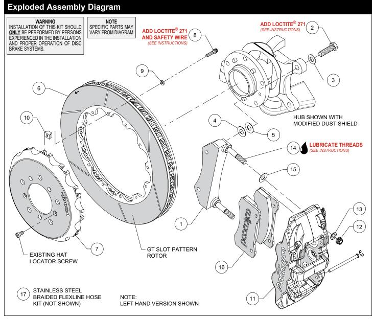
Figure 1. Typical Installation Configuration
