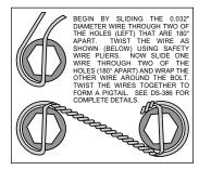
Figure 3. Safety Wire Diagram
