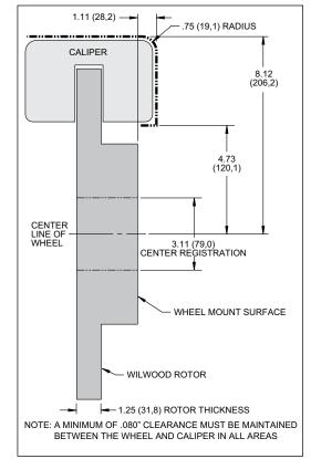
Figure 2. Wheel Clearance Diagram
