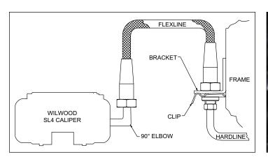
Figure 3. Brake Line Diagram
