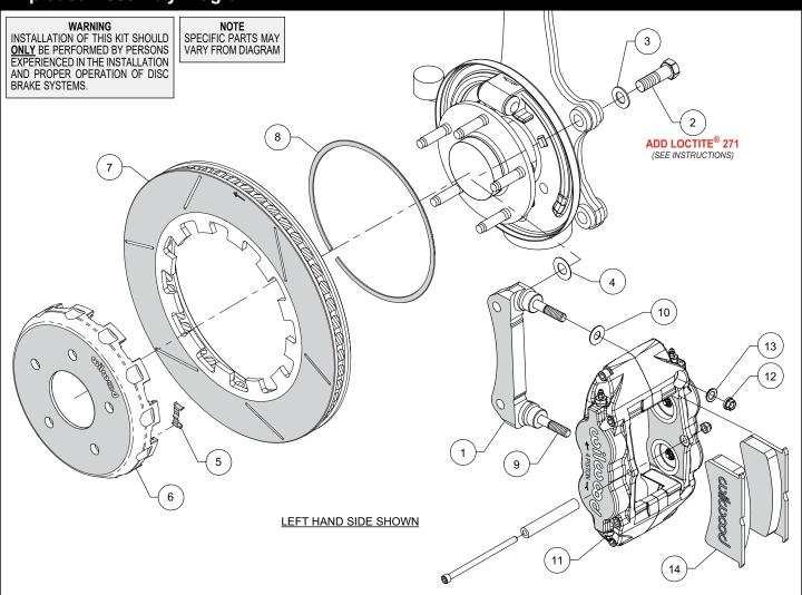
Figure 1. Typical Installation Configuration
