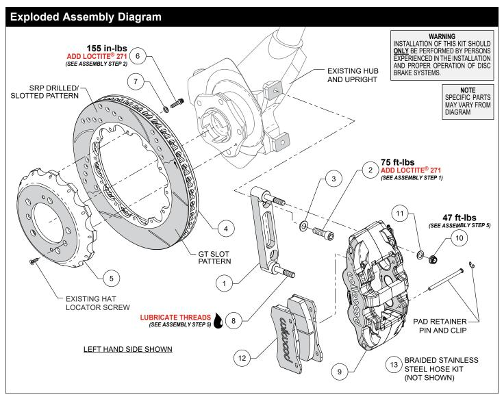
Figure 1. Typical Installation Configuration
