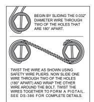
Figure 3. Safety Wire Diagram
