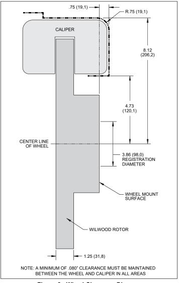
Figure 2. Wheel Clearance Diagram
