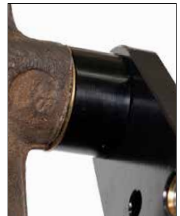
Photo 3 Spacer for disc spindle (.700")
