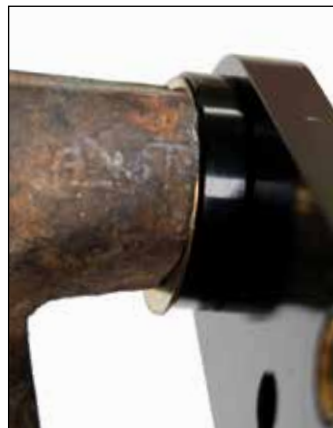
Photo 2 Spacer for drum spindle (.250")
