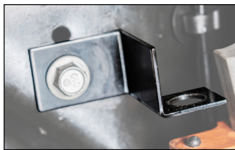
Photo 6 (Brake line chassis bracket mounting)
