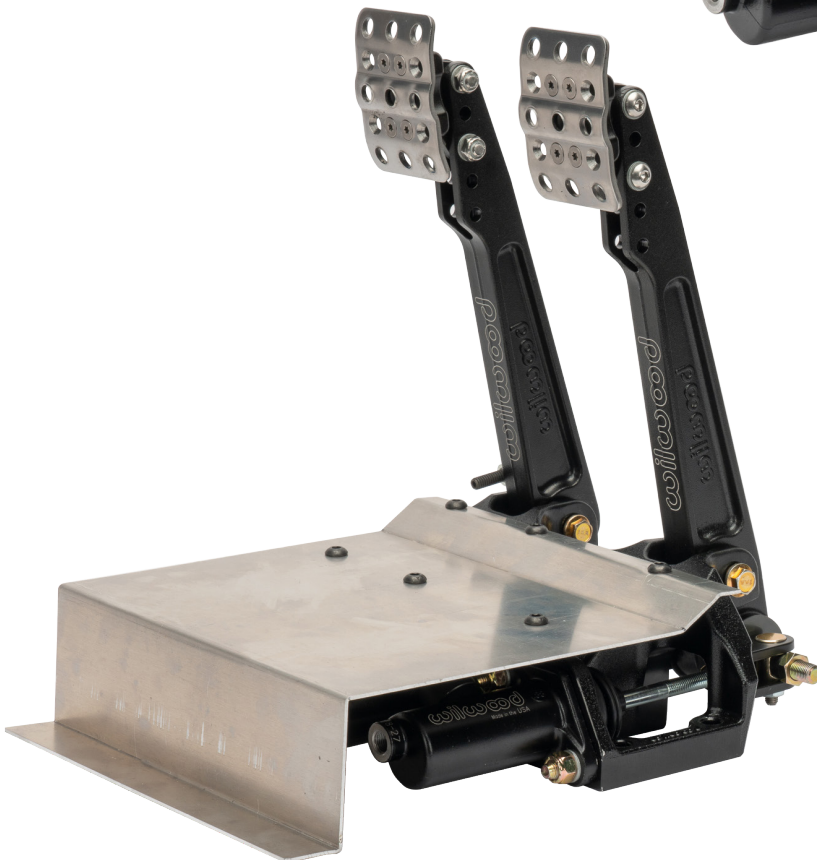
Photo 2. Reverse Mount Dual Pedal Assembly, 5.25:1 to 6.00:1 Adjustable Ratios, (p/n 340-17803), shown with master cylinders and false floor, not included
