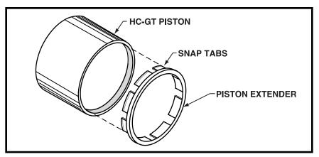
P/N 300-5069: 1.50" Diameter Piston Extender - Use with HC-GT Piston P/N 200-4833 P/N 300-5070: 1.75" Diameter Piston Extender - Use with HC-GT Piston P/N 200-4834
