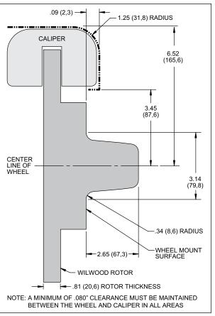
Figure 2. Wheel Clearance Diagram
