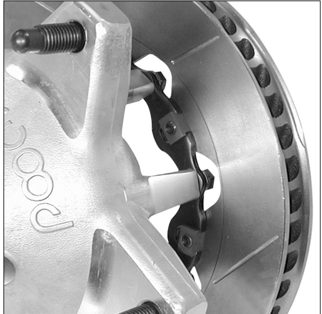
Wide 5 Racing Hub Floater Assembly Showing T-Nut Placement with Rotor and Mounting Plate
