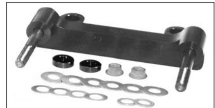
Typical Caliper Mounting Bracket
