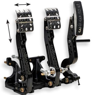
**Tru-Bar Adjustable Brake, Clutch, Throttle**
