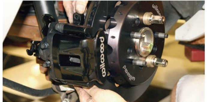
The rotor to caliper centering was checked to make sure it was lined up properly. The shims included in the kit can be used to make small adjustments.
