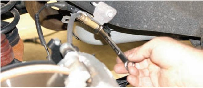
Disassembly of the rear brakes was started by disconnecting the steel line from the rubber line as seen here. After the lines were disconnected, the bracket was removed from the inner fender well.
