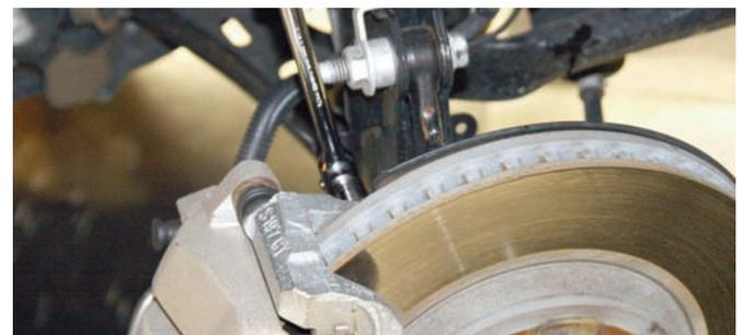
Using a socket wrench and the appropriate size socket, the two bolts and washers that fasten the caliper to the bracket were disconnected. This is a heavy cast iron caliper, so the Wilwood brake kit with aluminum calipers will lower the weight of the car.
