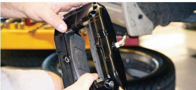
The pads were installed in the caliper and they were secured with the bridge bolts. This kit is using the BP-10 Smart Pads. Here you can also notice the brake line fitting in the caliper body that was installed with Teflon tape wrapped around the threads.
