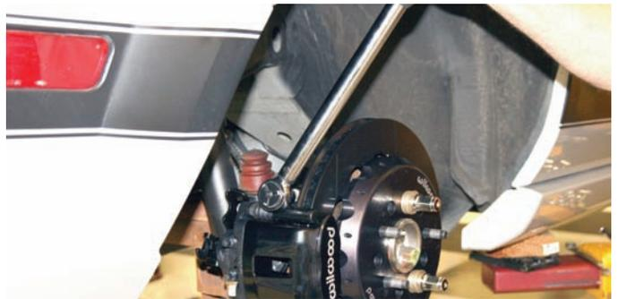
The correct amount of shims and washers were installed to get the caliper centered over the rotor. Here the caliper mounting nuts were coated with Loctite 271 and were tightened to 30 ft-lbs.
