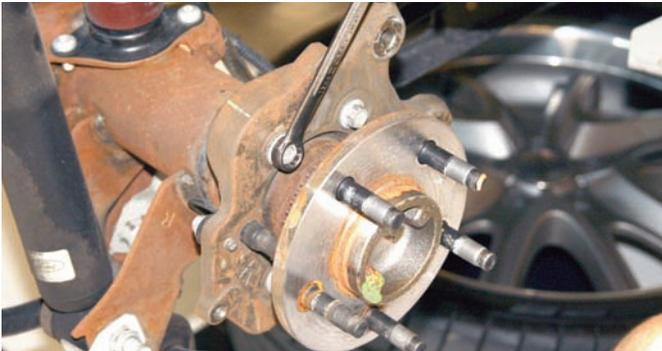
This original caliper bracket bolt was removed because it will be used to connect the Wilwood intermediate caliper bracket.
