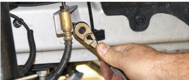
The original frame bracket, where the steel line mates to the rubber line, was disconnected so that it can be modified to work with the Wilwood braided steel Flexline.
