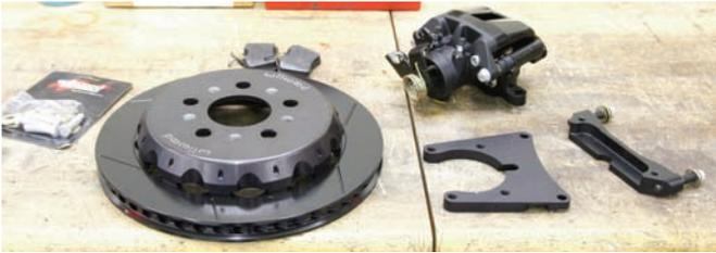
The rear rotors, caliper and caliper brackets were placed on a bench prior to installing the parts on the car. The rotors were assembled by connecting the hat to the rotor using the 1/4-20 bolts in the kit. The bolts were coated with Loctite 271 and then they were tightened in an alternating sequence to 103 in-lbs. After the bolts are tight they were safety wired using standard 0.032-inch diameter stainless steel safety wire.
