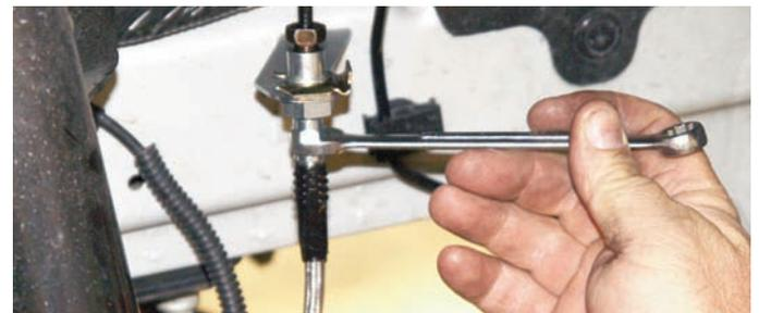
The Wilwood braided steel Flexline was routed between the bracket on the frame and the fitting on the caliper, making sure that it doesn't interfere with any moving parts.
