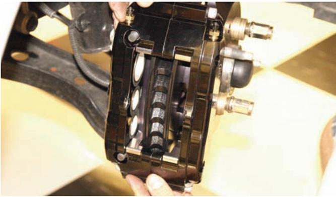
The caliper was connected to the bracket to see if it was centered properly. Using the shims in the kit, the centering was adjusted and that number of shims and washers were used when the bracket was bolted on for the final time.
