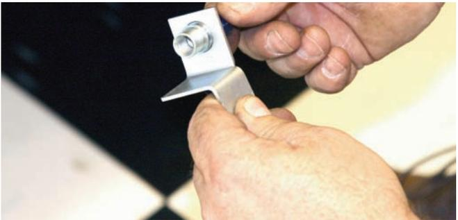
Similar to the way the front bracket was modified, this one was opened up so that it would accept the fitting shown here. After that was finished the bracket was bolted back into the original location with one side of the fitting connected to the steel line.
