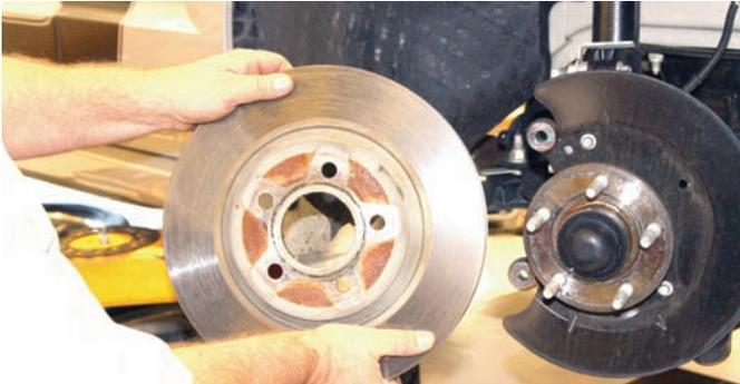
After the removal of the caliper, the rotor was disconnected from the hub assembly to reveal the hub and upright. Sometimes you will have to tap the rotor with a rubber mallet to break it loose.
