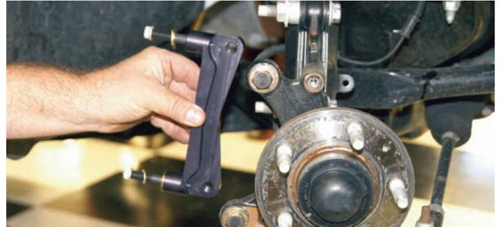
The Wilwood caliper bracket was bolted to the original caliper mounting holes in preparation for getting the proper caliper to rotor spacing.
