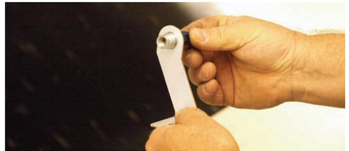
The hole in the bracket was opened up so that this fitting could be installed. It will be held in place with a brake line clip.
