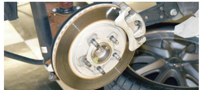
The wheels were reinstalled and the front of the car was lowered. After the front of the car was on the ground, the rear of the car was raised and jack stands were installed under the differential. The wheels and tires were removed to reveal the rear brakes.
