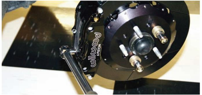
After it was determined that the caliper was positioned correctly, the mounting nuts were tightened to 35 ft-lbs. The wheels and tires were reinstalled and the front of the car was lowered.
