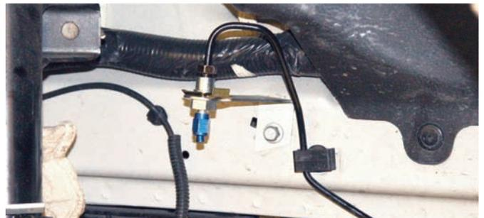
Here is the bracket with the steel line and fitting installed, and ready for the braided steel Wilwood Flex line. Here you can see the brake line clip that holds the fitting in place.
