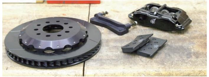
The rotor and the hat were bolted together using the 1/4-20 bolts and corresponding washers in the kit. The bolts were tightened to 85 in-lbs and then they were safety wired using standard 0.032-inch diameter stainless steel safety wire. The rotor, caliper, caliper brackets and pads were placed on a bench prior to installation for easy access.
