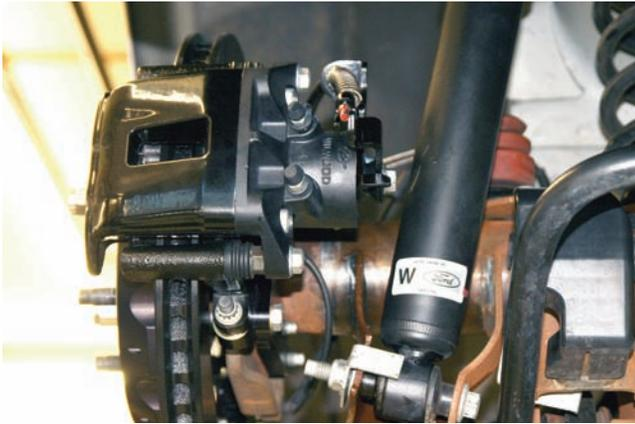
This CPB caliper is a combination unit that uses hydraulics for the brake pressure and an internal mechanical lock for the parking brakes. The parking brake cable was connected to the lever on the side.
