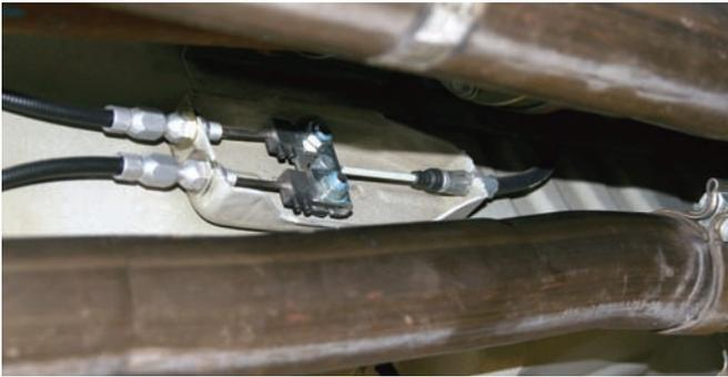
The parking brakes for the Mustang were connected using the Wilwood Parking Brake Cable Kit. This system will use a combination of original parts in conjunction with the Wilwood part number 330-9371 universal kit.
