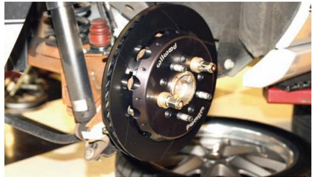
The rotor was installed and it was secured with two lug nuts. This was done to check the rotor to caliper centering.
