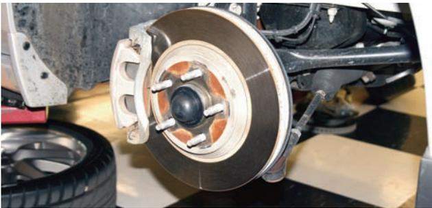
The front of the Mustang was raised using the floor jack and then jack stands were placed under the car for safety. The wheels and tires were removed to access the original Mustang brakes. The Ford rotors and calipers are going to be removed in preparation for the new brakes.
