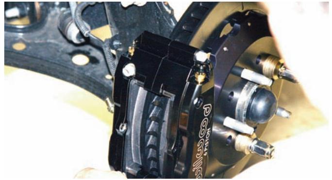
The caliper was placed on the bracket so that the rotor centering can be checked one more time. The curve of the brake pads should also line up with the curved edge of the rotor, and as you can see here, they are perfectly lined up.
