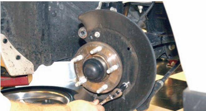
After the rotor was removed, the bolts that secure the dust shield to the spindle were disconnected using a small socket wrench.
