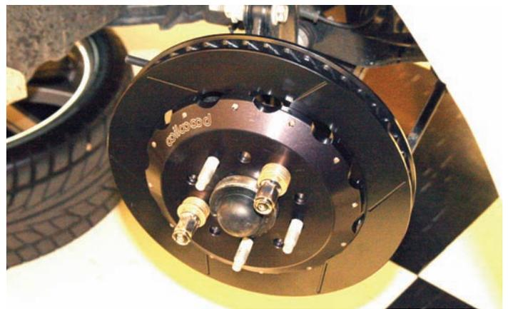
A couple of lug nuts were used to secure the rotor to the hub assembly so that the rotor to caliper centering could be studied. Since this is a top mounted caliper, the centering can be adjusted by placing shims between the caliper bracket and Ford bracket.
