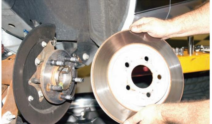
The rotor was removed from the rear axle flange as seen here. Some light tapping with a rubber mallet will help loosen the connection.
