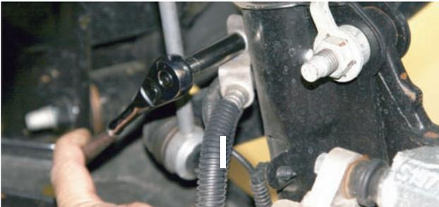
The original rubber brake lines were removed in preparation of installing the Wilwood Flexlines. The bracket by the strut was disconnected and it will be modified to work with the Wilwood lines.
