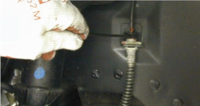
Using a line wrench, the hard line was disconnected from the flexible line. This bracket will also be used to mount the Wilwood brake hose.
