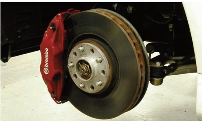
Here are the front brakes that come standard on the car. The Brembo brakes are better than what you will find on other Mitsubishi products but they are heavy and the car's stopping power and handling can be improved.
