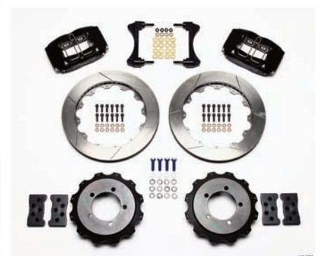
The Wilwood Engineering part number 140-9285 front brake kit comes with 14-inch diameter slotted rotors, aluminum hat adapters, Billet Narrow SL6 Radial Mount six-piston calipers, aluminum caliper brackets, BP-10 Smart Pads, and all of the hardware required to finish the installation.
