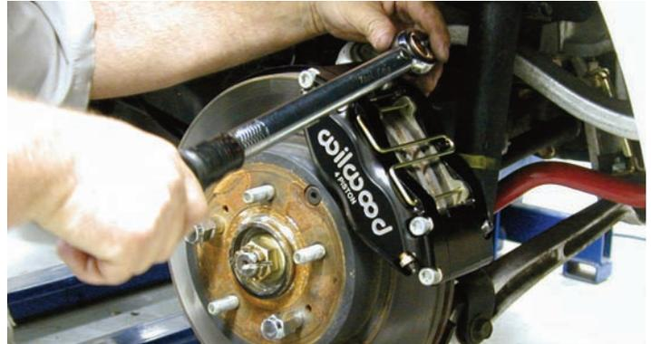
After the caliper was installed and the rotor was centered, the 0.057-inch thick washers were installed and the 3/8-24 self-locking hex head nuts were tightened to 35 ft-lbs.
