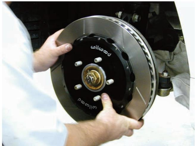
After the bracket was in place, the rotor was lifted and placed on the hub assembly as seen here. The aluminum hat was connected to the rotor using the bolts and washers in the kit. The bolts were coated with Loctite 271 and then they were tightened to 85 in-lbs in an alternating sequence using an inch-pound torque wrench.
