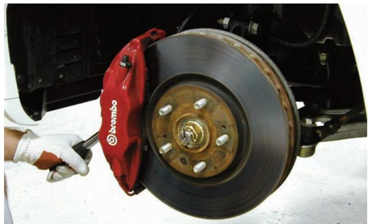
Using a breaker bar and the correct size socket, the two bolts securing the caliper to the bracket were disconnected.
