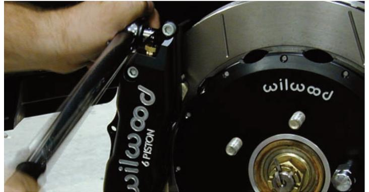
After the two self-locking nuts were snug, they were tightened to 35 ft-lbs using a foot-pound torque wrench.
