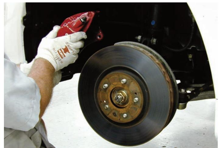
After the caliper bolts were disconnected the caliper was removed from the assembly.
