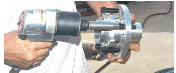
The Wilwood aluminum hubs have two sets of holes, one for the Ford pattern and another for the Chevy pattern. Because of this, you have to pick the correct bolt pattern and then install the lug studs. The studs should be tightened to 77 ft-lbs using a foot-pound torque wrench.
