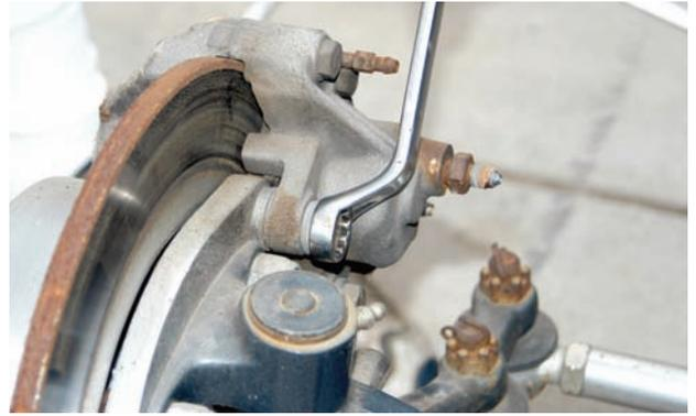
The two caliper bolts were removed next, and then the caliper was removed from the brackets.
