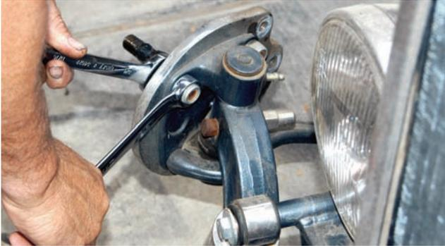
The disc brake caliper brackets were removed from the spindle. The top uses nuts and bolts and the lower bolts actually attach to the steering arms.
