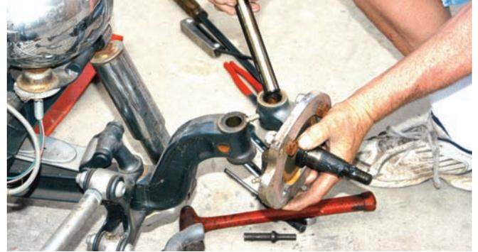
After the kingpin retaining bolt was removed, the kingpin could be pulled out of the axle. The kingpin also connects to the spindle, so it was also removed.
