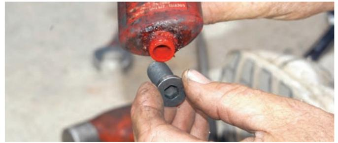
The bolts that secure the bracket should be installed with Loctite. These are high strength Allen bolts.
