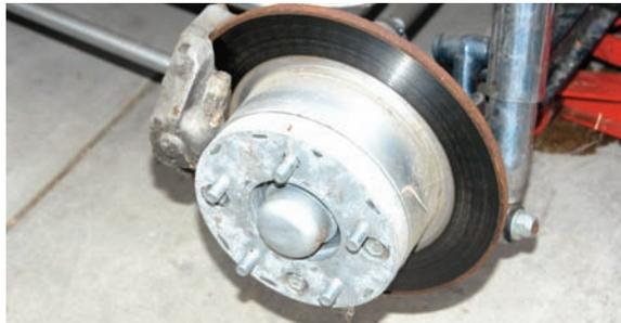
Volkswagens used a four-lug bolt pattern so the first thing that had to be done was get an adapter that would change the brakes to a Ford or Chevy pattern. Here's the original VW brake system with the adapter installed.
