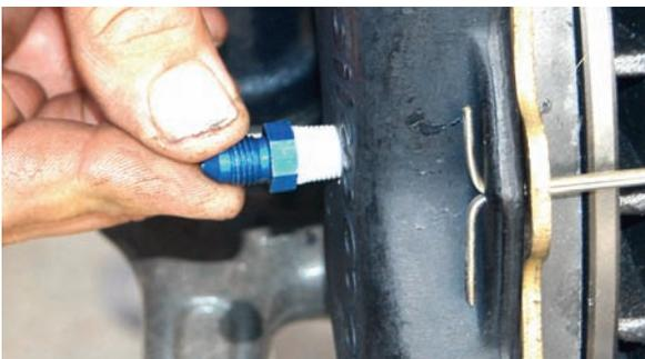
The kit comes with an AN fitting that should be secured to the caliper. It should be installed with some Teflon tape to prevent leaks.
