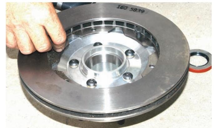
The rotor bracket is secured to the hub with five Allen bolts. The rotor is attached to the adapter with six bolts. All of the bolts should be coated with Loctite 271 and then the hub to rotor bolts should be tightened to 180 in-lbs using an inch-pound torque wrench. The hub to rotor bolts should be tightened to 22 ft-lbs using a foot-pound torque wrench.
