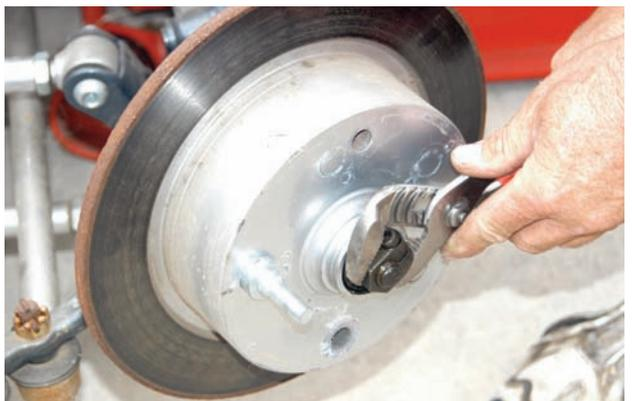
After the Allen bolt was loose, the spindle nut was removed using large channel lock pliers.
