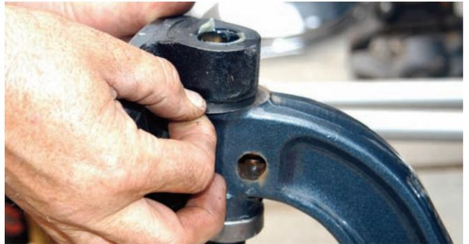
The new Total Cost Involved Engineering spindle was set in place. The spindle uses a large bearing underneath. If the spindle seems a little loose, shims can be used to tighten it up. In this case a thin shim was used.
