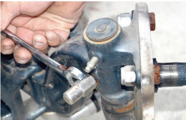
The large acorn nut on the side of the axle connects to the kingpin retaining bolt. It was removed in preparation for kingpin removal.
