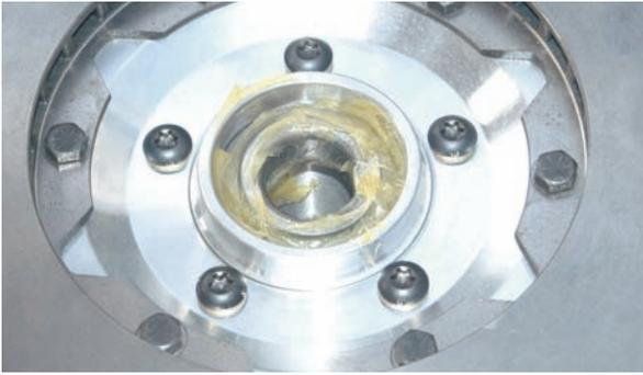
The kit comes with all of the bearings so the large bearings were packed and they were installed in the rear side of the rotor. The races for the rear and front bearings come installed in the hub assembly.
