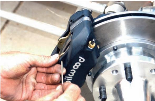
The brake pads are secured with a large retaining pin. Bend the ends so the pin doesn't come out but make sure it can come out when the pads need replacement.
