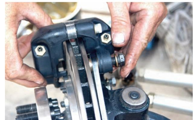
The aluminum calipers were installed with two case hardened bolts. If you look close, the bolts are drilled for safety wiring. It's important for the calipers to be centered over the rotor so shims have been included in the hardware package.
