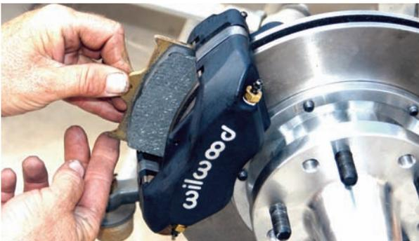
The pads can now be installed in the caliper. We really shouldn't have to say this, but the lining should be pointing toward the rotor.
