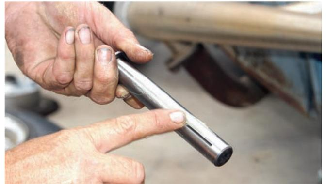
New kingpins are being used and they were greased before being installed. The new kingpins will tighten up the front suspension.
