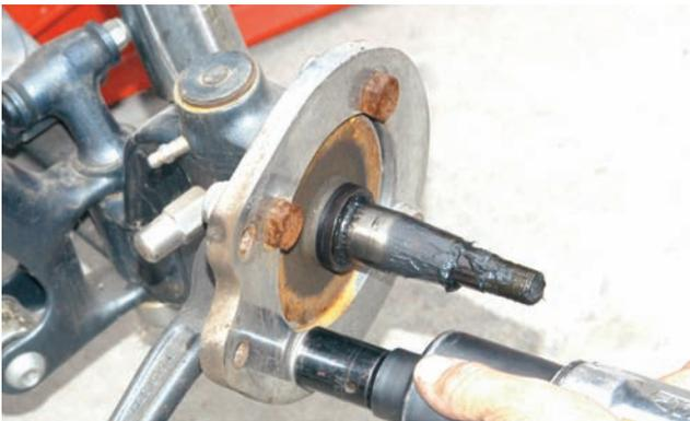
The bolts securing the steering arms were removed with an impact gun.
