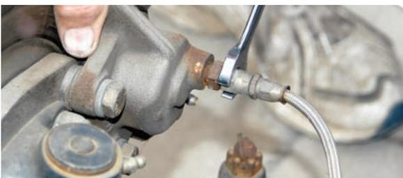
The brake line to the caliper had to be removed. This was done with a line-wrench to avoid stripping the fitting. The brake line will be retained and used with the new calipers. After the line was disconnected it was plugged to stop the fluid from leaking.
