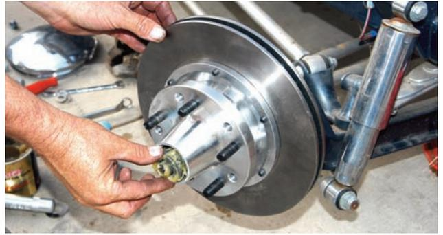
The rotor was placed on the spindle and then the small front bearing was thoroughly greased and was installed in the front of the hub. That was followed with the large washer and the spindle nut.
