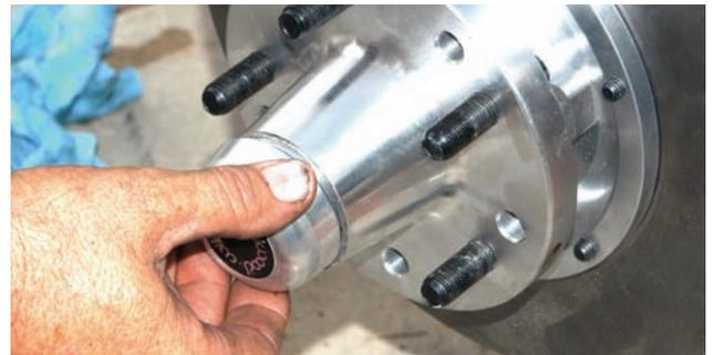
The Wilwood grease cap was installed to finish off the rotor installation.
