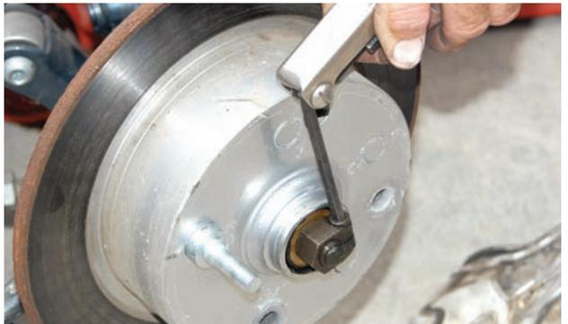
Although many American spindle bolts are secured with a cotter key, the Germans feel that it would be better to use an Allen lock bolt. Here the Allen lock is being loosened so that the spindle nut can be removed.
