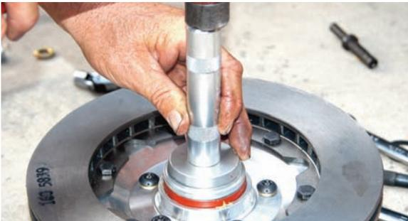
Using a grease seal installation tool, the seal was set in place. One or two hammer hits and the seal is in place and level with the rotor.
