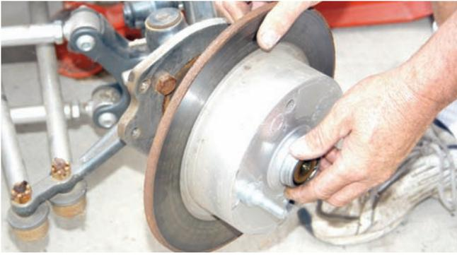
After the Allen bolt was loose, the spindle nut was removed by hand and then the rotor was removed from the spindle.
