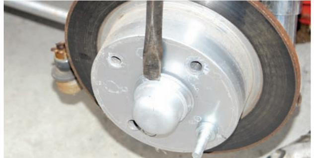
The grease cap was removed from the disc brake rotor. This cap was removed with a large screwdriver used as a pry bar.
