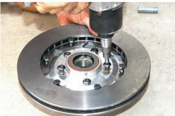
The hub bolts were finger tight so they were tightened with an impact gun followed by the inch-pound torque wrench. They should be tightened to 180 in-lbs.
