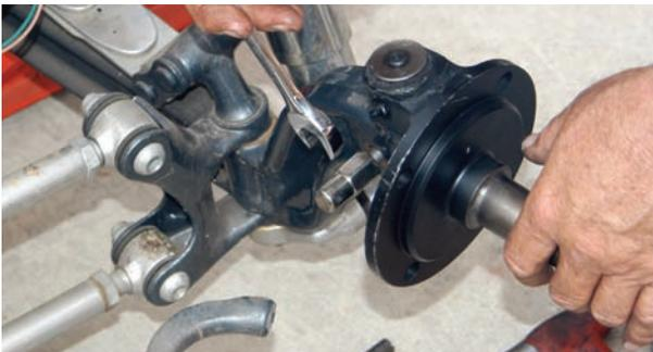
The nut was installed on the kingpin retaining bolt and then it was secured. It's a good idea to install a little Loctite.
