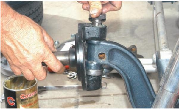
The upper felt washer and retainer were installed on the kingpin and then it was installed through the spindle and axle. The small notch in the kingpin should be lined up with the hole in the axle.
