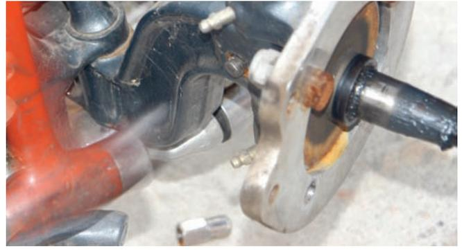
The kingpin retainer was loosened by tapping it with a hammer. Some WD40 was sprayed on first.
