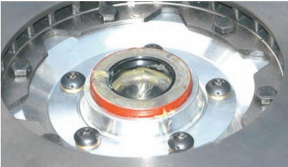
The next step is to install the grease seal that also comes installed in the kit. Here the seal is resting on the seal opening.
