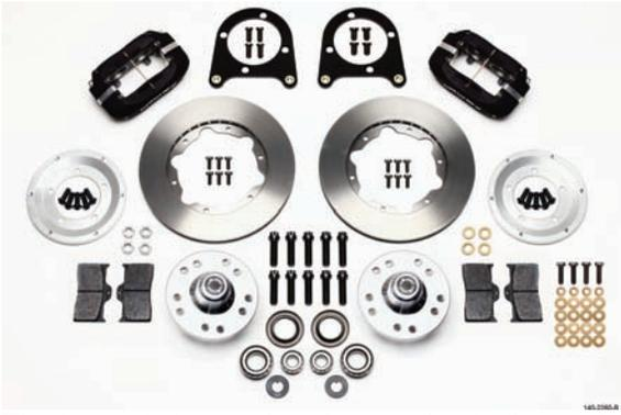
The hot rod shop ordered a set of spindles and kingpins from Total Cost Involved Engineering (not shown) and the brake installation kit from Wilwood Engineering. The part number 140-2260 brake kit came with the disc brake rotors, aluminum calipers, and aluminum hubs with bearings, caliper brackets and all of the hardware needed to complete the installation.
