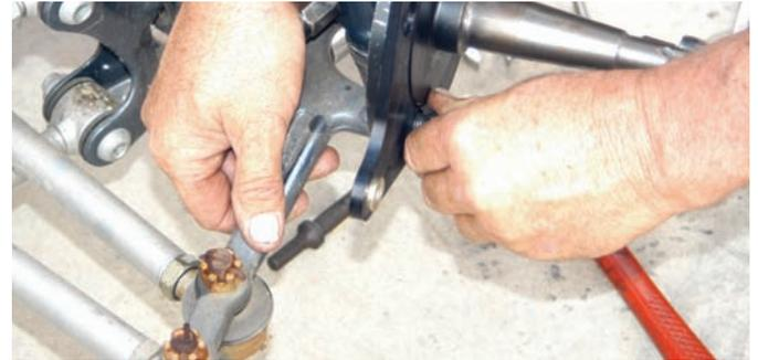
The two lower bolts secure the steering arms. It is very important to make sure these bolts are tight and won't back out so coat them with Loctite.
