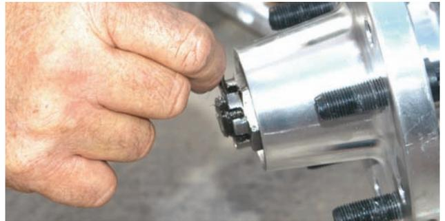
The hub assembly and rotor are secured with a large castle nut. A castle nut has to be used with a cotter key. The nut should be tight but not enough to create binding in the bearings.
