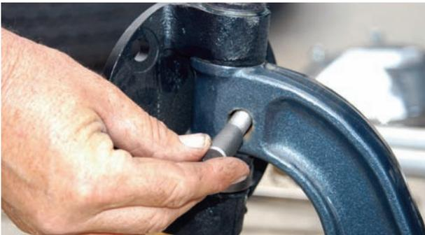
The kingpin retaining bolt was installed in the axle. This is a tapered retainer nut that keeps the kingpin from turning in the axle.
