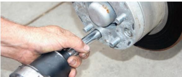
Removing the thick adapter plate started the installation. It is secured with three bolts and one of the VW lugs.
