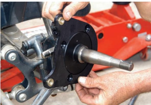
The Wilwood caliper bracket was installed on the spindle. The part of the bracket that secures the caliper faces toward the back of the car.
