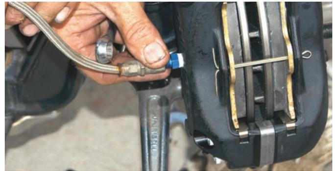
An aircraft line was used on the old system so we were able to connect it to the new caliper. It should be very tight to prevent leaks.
