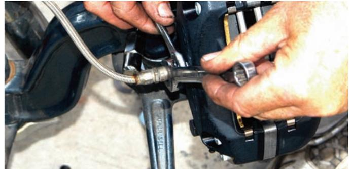
Using two wrenches, the brake line is tightened. After the hoses are installed the brakes will need bleeding to get the system working properly.
