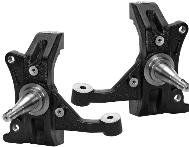
Wilwood 2.00" Drop ProSpindles for C1500 Pickup Trucks P/N 831-15933 (1988-1998)
