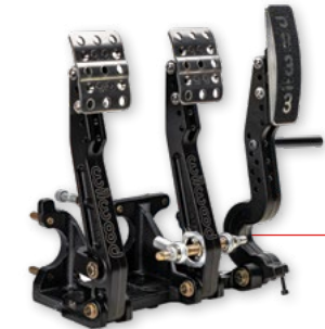
OFFSET CLUTCH/BRAKE ADJUSTABLE RATIO
