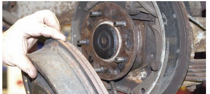
After the linings were backed off just a little, the brake drums were removed to access the brake assembly and backing plate.
