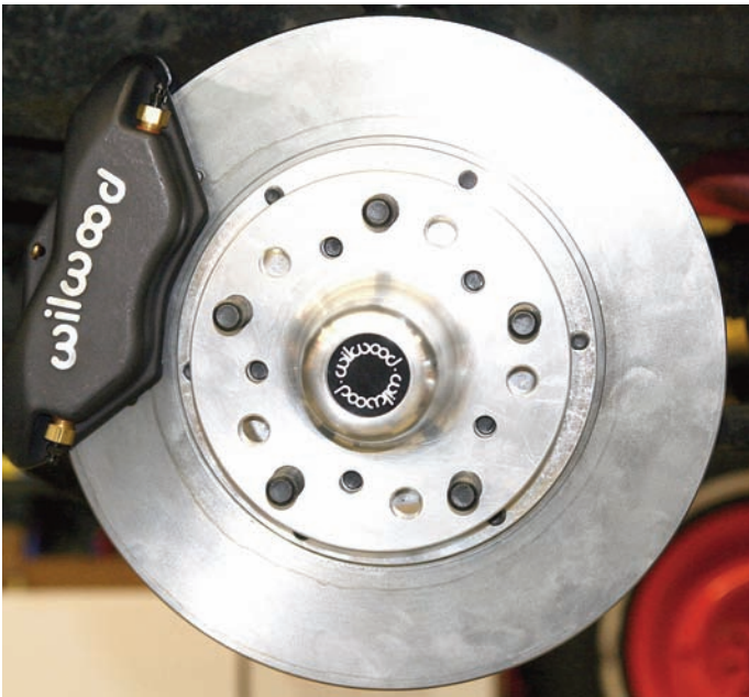
Here is the finished brake assembly with the Caliper mounted and ready to go. Before that is done the brake line was hooked up.
