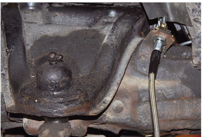
The other end of the braided steel line should be run to the frame bracket where it mates with the car's hard line.
