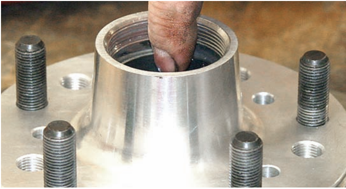
After the rear bearing was installed, the rotor was installed on the spindle. The small inner bearing race was coated with grease prior to installation.
