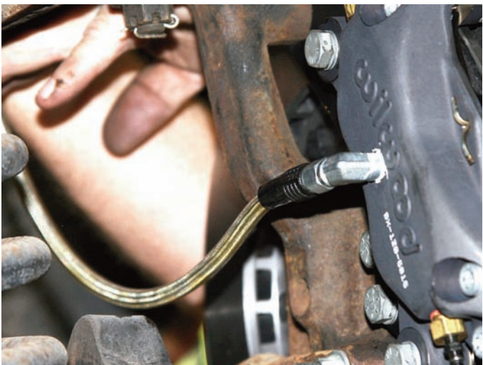
The braided steel brake line was connected to the caliper inlet fitting. The connection should be made with a line wrench so that it can be tightly connected.
