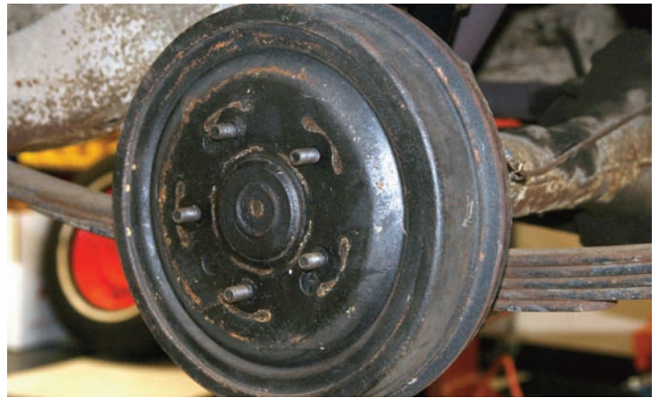
Now it's time to handle the rear brakes. The brake linings should be backed off just a little to make it easy to remove the brake drum.
