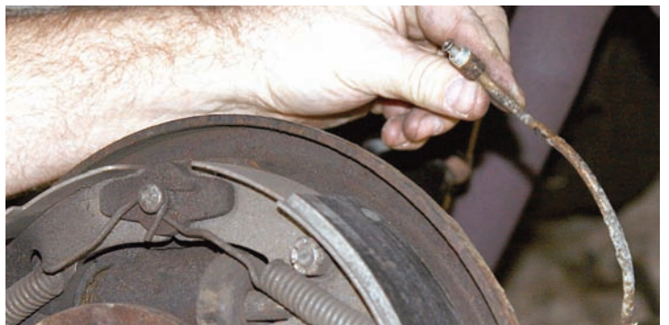
Using a line wrench, the brake line was removed from the wheel cylinder assembly. The brake lines and wheel cylinders look like original equipment.
