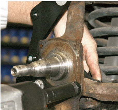
The bracket was lined up with the large spindle hole and then the bolt was installed with a ratchet wrench and an Allen head socket.
