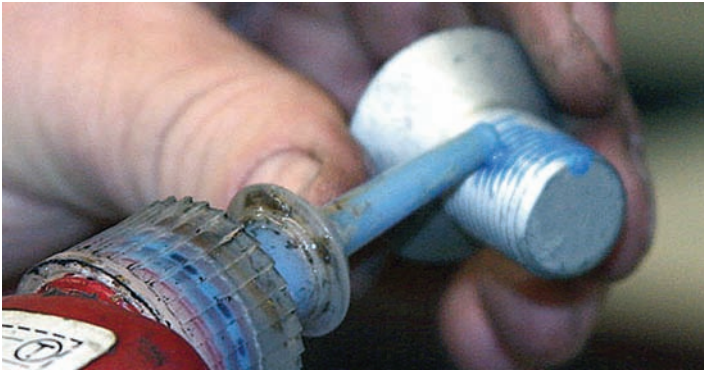
A large Allen head bolt connects the upper portion of the bracket to the spindle. Before it was installed, it was coated with Loctite 271.
