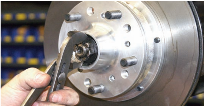
The large flat washer was installed and then the spindle nut was screwed into place. The nut was tightened until it was snug, but not overly tight. If the nut is too tight it will cause premature bearing failure.
