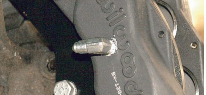
The caliper inlet fitting threads were coated with Teflon tape and then it was screwed into the caliper.
