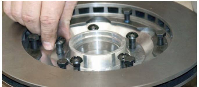
The aluminum adapter was bolted to the hub assembly using the Allen bolts in the kit and then the rotor was bolted to the adapter plate using the hex head bolts in the kit.
