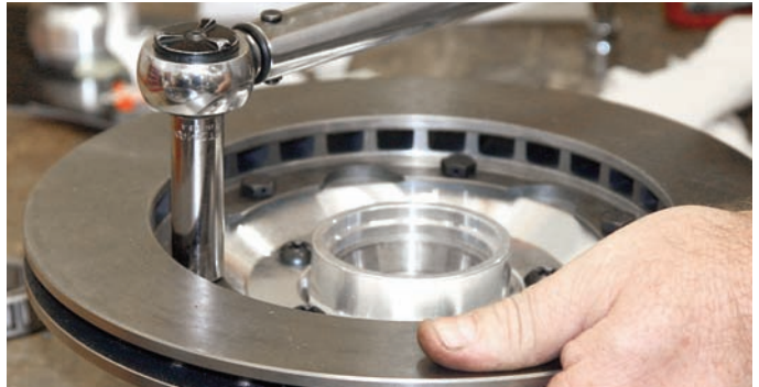
All of the rotor assembly bolts were coated with Loctite 271 and the hub to rotor bolts were tightened to 180 in-lbs using an inch-pound torque wrench. The rotor-to-adapter bolts were tightened to 35 ft-lbs using a foot-pound torque wrench.
