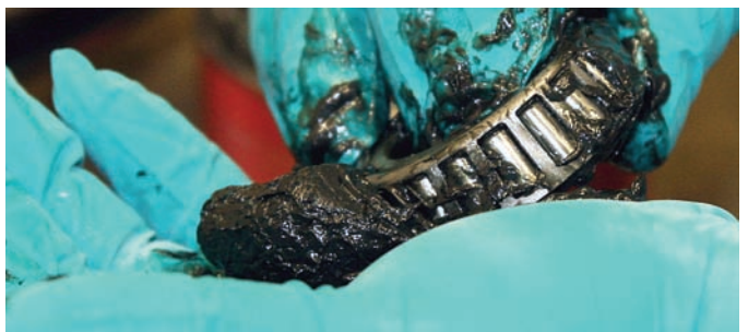
All of the bearings were packed with high temperature disc brake bearing grease. The large bearings were installed in the rear of the hub and then the grease seal was installed.
