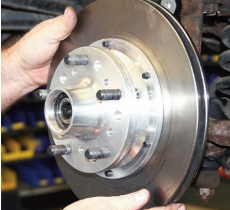
After the rear bearing was installed, the rotor was installed on the spindle. The small inner bearing race was coated with grease prior to installation.
