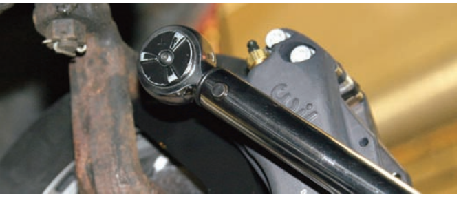
Here the caliper bolts are being tightened to 35 ft-lbs using a foot-pound torque wrench.
