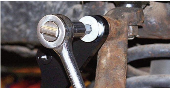
The bracket was lined up with the large spindle hole and then the bolt was installed with a ratchet wrench and an Allen head socket.
