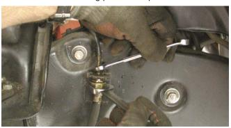
Before the backing plate could be removed, the brake hose had to be disconnected from the steel line. Here the connection is being disconnected with an openend wrench and a line wrench.
