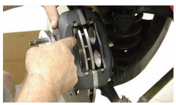
After the rotor was in place, the caliper was connected to the caliper bracket using the bolts, washers and shims in the kit. The caliper was bolted to the bracket and then the caliper to rotor centering was checked. Shims are used to get the centering perfect.
