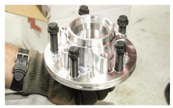
Using the correct Chevy 5 on 4 3/4-inch spacing, the lugs were installed into the aluminum hub assembly. The lug studs were tightened to 77 ft-lbs.
