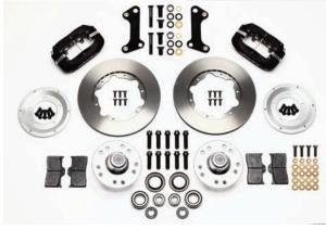
The front disc brake kit comes with the rotors, calipers with pads, caliper brackets, and all of the hardware required to complete the installation. A full set of instructions is also included to show you how the installation is done.
