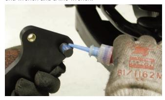
After the backing plate was removed, the caliper bracket could be installed. The bolts were coated with Loctite 271 before installation.
