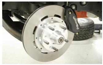
Here is the front brake assembly after the installation was completed. This should be a huge improvement over the original Chevy drum brakes in overall stopping and in bad weather conditions.
