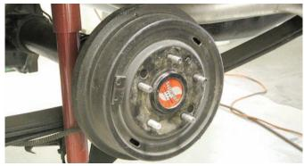
The front wheels were bolted onto the disc brakes and the front of the car was lowered so the rear of the Camaro could be elevated. This Camaro features a strong running small-block Chevy engine so it is equipped with a 12-bolt Chevy differential. Drum brakes are used at the rear so Wilwood rear disc brakes will get this Camaro stopping efficiently.
