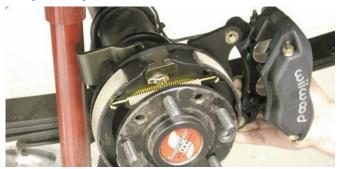
The caliper was held up to the bracket to check the bolt spacing. Everything was looking good but the caliper couldn't be installed until the rotor was connected.
