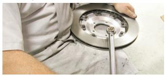
The rotor adapter plate to rotor bolts were tightened to 180 in-lbs and then they were safety wired in place. A safety wire diagram can be found in the instruction sheet.
