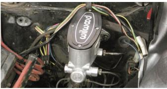
The master cylinder is filled with Wilwood Hi-Temp 570 racing brake fluid and it is ready for bleeding. This Wilwood master cylinder works great and it is also a nice appearance addition to any vehicle.
