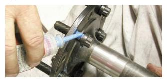
The lug studs were coated with Loctite 271 and then they were screwed into the holes. The studs were tightened to 77 ft-lbs.
