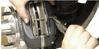
The brake pads are secured with a long cotter key. The ends were bent enough to hold the key in place but not too much because the key will have to be used again when the pads are replaced in the future.
