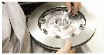
The hub assembly was connected to the rotor adapter plate using the bolts supplied in the kit. Using a torque wrench, the bolts were tightened to 22 ft-lbs and then they were safety wired.
