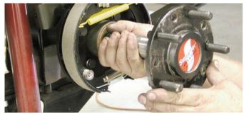
Following the installation of the internal parking brake mechanism and caliper mount, the axles were reinstalled into the axle housing. Replace all of the parts in the center section and then install the differential cover using a new gasket.
