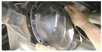
The axles have to be removed from the differential so the differential cover was removed to access the C-clips. A drip pan was placed under the axle, the cover bolts were disconnected and then the cover was carefully lifted and removed from the axle. Before this is done, it would be advisable to have another pan gasket and some silicone ready for installation.
