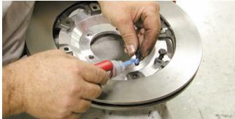
The rotor adapter plate was connected to the rotor using the bolts supplied in the kit. Before the bolts were installed they were coated with Loctite 271.
