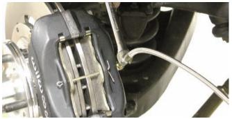
Using an open-end wrench, the part number 220-7056 Wilwood Flexline was connected to the caliper.
