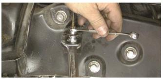
The Wilwood Flexline was connected to the original steel line using an open-end wrench. The Flexline was secured with an open-end wrench and the steel line was tightened with a line wrench after the initial connection was made.
