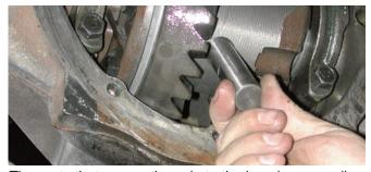
The parts that secure the axle to the housing were disconnected so that the axles could be removed. If you have a shop manual for your car, use it as a guide for axle removal.
