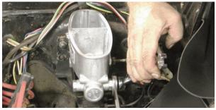
Using a large and small line wrench, the original brake line was connected to the new master cylinder.
