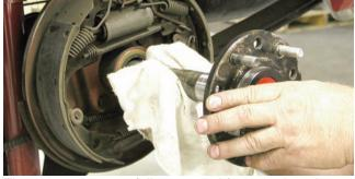
The axles were carefully removed from the housing making sure you note which side they came out of. Many differentials have a short and a long axle.
