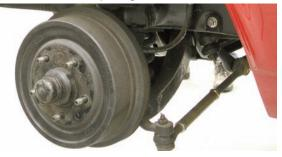
This '67 Camaro came from the factory with standard four-wheel drum brakes. Disc brakes were optional in 1967 and they were primitive. We are updating this Camaro with a Wilwood part number 140-2285-B disc brake kit that can be installed on disc or drum brake spindles.
