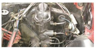
In 1967 all American cars had to have a dual master cylinder for safety, so this Camaro had a non-power master cylinder designed for drum brakes. This original master cylinder will have to be changed to a Wilwood dual master cylinder designed for disc brakes front and rear.
