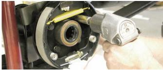
After the backing plate was removed, the axle flange was cleaned off with a wire brush and then the Wilwood caliper bracket and internal parking brake mechanism was installed using the same four mounting holes. The bolts were tightened with an impact gun and an openend wrench.
