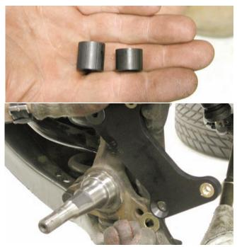
The caliper bracket was installed using the two spacers in the kit. The large spacer and a washer are used at the top connection and a small spacer and a washer are used at the lower connection.
