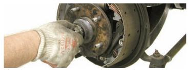
After the cotter key was removed, the spindle nut and large flat washer were disconnected with a large Crescent wrench and then the nut was loosened by hand. After the nut was disconnected, the hub assembly was removed. The nut and washer were retained for use later.
