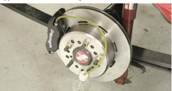
Here is the finished rear brake assembly and it certainly will be a nice performance addition to this '67 Camaro. After the bleeding procedure is finished the brakes will have to be bedded following the procedure outlined on the instruction sheet.
