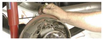
Using a line wrench, the original steel lines were disconnected from the wheel cylinders on both sides of the car.
