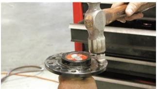
Wilwood hats center on ½-inch studs and Chevy uses 7/16-inch studs. You will have to take the axles to a machine shop and have the lug holes drilled and tapped for fine thread ½-inch lug studs.
