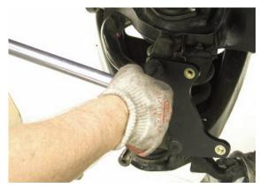
The upper bolt was tightened to 120 ft-lbs and the lower bolt was tightened to 77 ft-lbs. Because there are tolerance variations among spindles, it may be necessary to install a shim washer between the spacers and the bracket.
