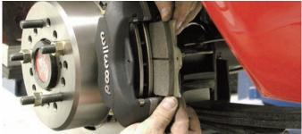
The rotor was installed and it was bolted to the axle. The caliper was connected to the bracket and then the caliper to rotor centering was determined. After the caliper was in alignment, the bolts were coated with Loctite 271 and then they were installed and tightened to 30 ft-lbs. After the caliper was centered, the BP-10 Smart Pads were installed.
