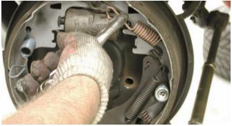
The springs that are connected to the special center bolt were removed. The center spring connection is also a bolt that fastens to the spindle.
