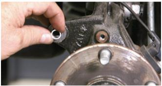
The former caliper mounting ears will have to be sleeved down slightly to the size of the Wilwood caliper bracket bolts.
