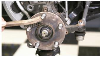
The hub assembly was thoroughly cleaned with a wire brush to remove any grease or debris.
