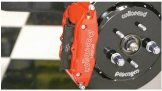
After the caliper was installed and tightened, the pads were installed from the top. After the pads were in place the caliper center bridge pad retainer bolt was installed.
