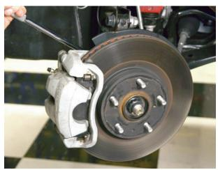
The caliper bolts were removed with a socket and a large breaker bar as seen here. This is a floating style caliper with a piston on one side applying the force. The six-piston caliper should be a big improvement.
