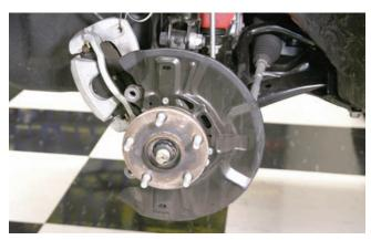
The original brake system uses this large dust shield that will have to be removed. You can also see the two ears that secured the original caliper
