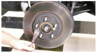
The rotor is secured to the hub assembly with a couple of small bolts. Here the bolts are being disconnected in order to remove the rotor from the hub.
