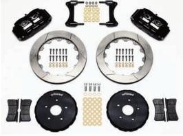
The toyoto was outfitted with a Wilwood part number 140-10752 disc brake kit that features Superlite 6R calipers and slotted 12.90-inch rotors with aluminum rotor adapters. The kit also comes with caliper brackets, BP-10 Smart Pads and all of the hardware required to complete the installation.
