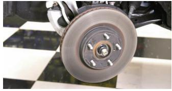
For now, the caliper was hung on a piece of coat hanger behind the rotor. The line will be disconnected a little later.
