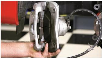
After the rubber hose was disconnected from the hard line, the caliper was removed from the car. Be careful not to get brake fluid on the car's painted surface because it works as good paint stripper.
