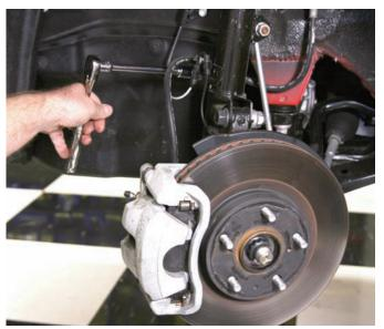
The small bracket that secures the brake hose to the inner fender was disconnected.
