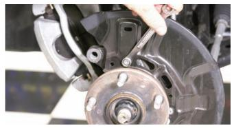
Using a small box-end wrench, the bolts that secure the dust shield to the spindle were removed.
