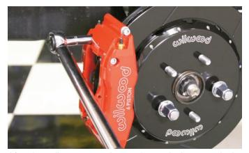
After the caliper was resting on the studs the 0.057-inch thick washers and self-locking nuts were installed and tightened. At this point the centering process was done and when it was finished, the caliper was tightened to 35 ft-lbs using a foot-pound torque wrench.
