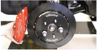
Carefully the large six-piston caliper was loaded onto the caliper mounting bracket.
