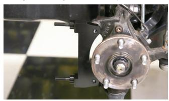
The caliper bracket was held against the original mounting ears and the bolts were installed hand tight.
