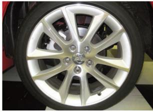
You can see the original calipers and disc brake system through the large windows in the stock Matrix wheel. The front of the car was elevated using a floor jack and then jack stands were placed under the car. After the front wheels were off of the ground, the lug nuts were disconnected with an impact gun and then the wheels were removed.
