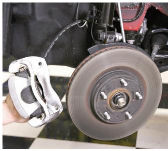
The caliper was removed from the assembly, but at this point it will remain hooked to the system.
