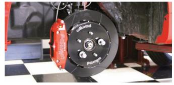
Here is the brake assembly finished and ready to go. At this point the brake system will have to be bled and the bedding process will have to be done to get the brakes working well and to full capacity.
