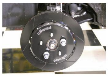
After the rotor was placed on the hub assembly, it was secured with two lug nuts in order to check the rotor to caliper centering.
