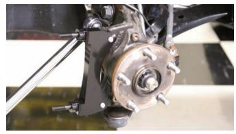
After the bolts were hand tight, they were tightened down with a large socket wrench. At this point they shouldn't be too tight because they may have to be loosened to add or subtract shims when the caliper to rotor centering is done. After the centering is complete, the bolts should be coated with Loctite 271 and tightened to 42 ft-lbs using a foot-pound torque wrench.
