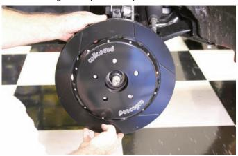
The hat was attached to the rotor using the 12 bolts and washers in the kit. The small bolts should be coated with Loctite 271 and then they should be tightened in an alternating sequence to 85 in-lbs using an inch-pound torque wrench. After the bolts were tight they were safety wired using the safety wire diagram in the instruction sheet. The completed rotor was installed on the hub assembly.
