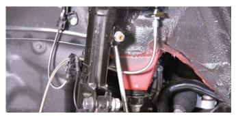
At this point the Wilwood part number 220-10803 hose assembly was installed. The hose runs from the bracket and hard line on the frame to the caliper assembly making sure the line is away from any moving parts.
