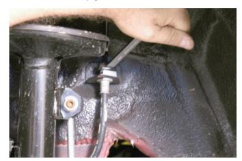
The rubber line was disconnected from the hard line using a line wrench. This connection is located on the inner fender well behind the strut.
