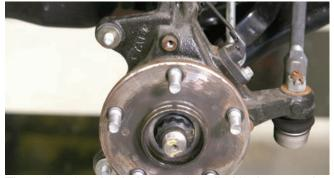
The caliper bracket bolts were installed in the mounting ears. There should be a washer on the outside and a 0.016-inch thick and a 0.030-inch thick washer between the original mounting ears and the caliper bracket.
