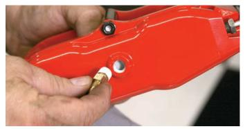
Here the caliper inlet fitting is being attached to the caliper. Before the installation, the threads were wrapped with Teflon tape.
