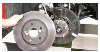
After the bolts were loose, the rotor was removed from the assembly. The rotor is in good condition so it can be stored with your other swap meet parts.
