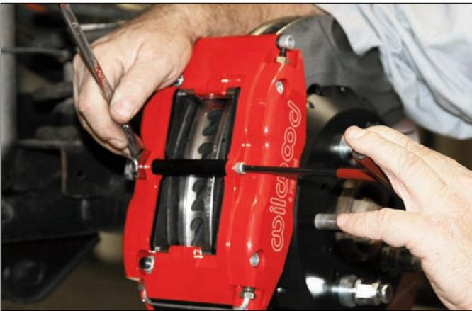
**Sequence 20:** After the pad height is set, install the center bridge pad retainer tub, bolt, and lock nut using an Allen wrench and open-end wrench. The lock nut should be snug without play in the bolt or tube. Be cautious not to over tighten. Then finalize the caliper mounting by torquing the caliper mounting lock nuts to 30 ft-lb.
