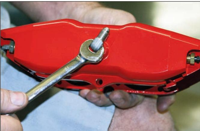
**Sequence 15:** Remove the protective sticker from the caliper fluid inlet. Coat the inlet fitting with PTFE thread tape and screw into the caliper with the 90° angle perpendicular to the length of the caliper toward the bleed screws.
