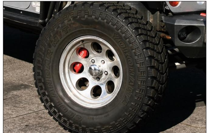
**Sequence 23:** Install the wheel and torque the lug nuts to manufacturer's specification. Ensure the wheel rotates freely without any interference. Bed in the brake pads and rotor in a safe location before general use driving.
