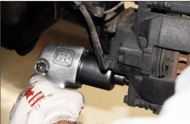
**Sequence 2:** Using a impact gun, or breaker bar and socket, break loose the caliper mounting bolts from the back side.
