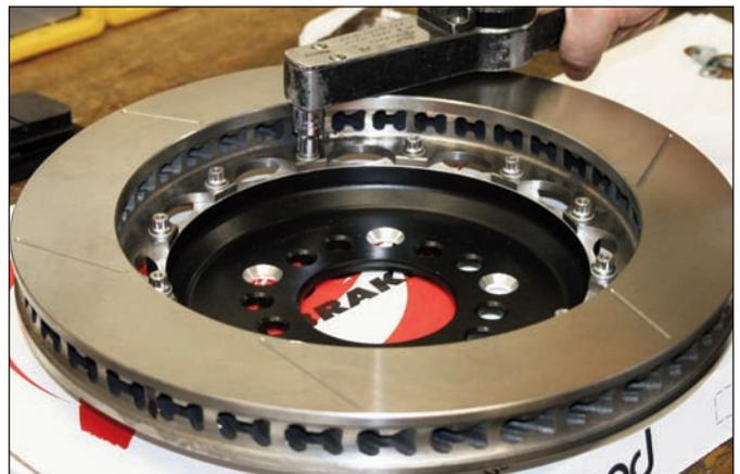
**Sequence 6:** Using an alternating sequence, torque rotor bolts to 155 in-lbs.
