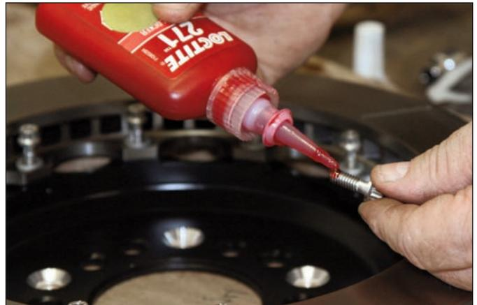
**Sequence 5:** Place one flat washer over each hole on the rotor mounting tabs. Apply red *Loctite*® 271 to the mounting bolts and slide through the washer and thread into the hat.
