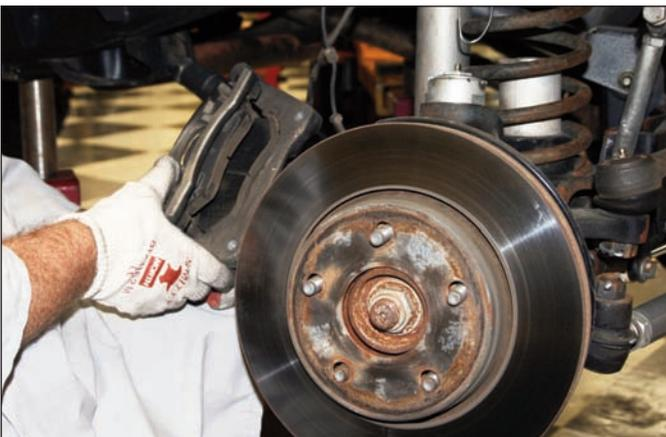
**Sequence 3:** Lift off and remove the caliper and hang off to the side using a piece of wire.
