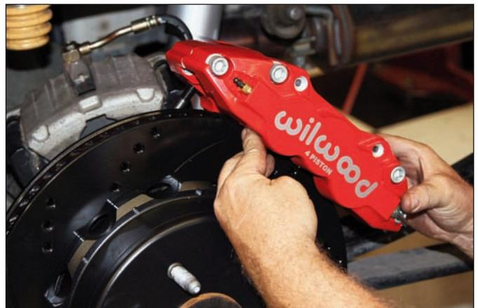
**Sequence 11:** This kit includes distinct right and left hand calipers. With the bleed screws pointing up, mount the caliper onto the bracket so that the largest pistons are at the rotor exit end of the caliper, in relation to the direction of rotor rotation.
