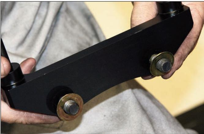
**Sequence 8:** Slide the original caliper mounting bolts through the caliper mounting bracket from the inboard side and place one washer on each bolt. Secure bracket to inboard side of caliper mounting ears. Temporarily tighten the mounting bolts. **NOTE:** The bracket must fit squarely against the mounting ears. Inspect for interference from casting irregularities, burrs, etc. Grind as necessary. Do not Loctite at this time.
