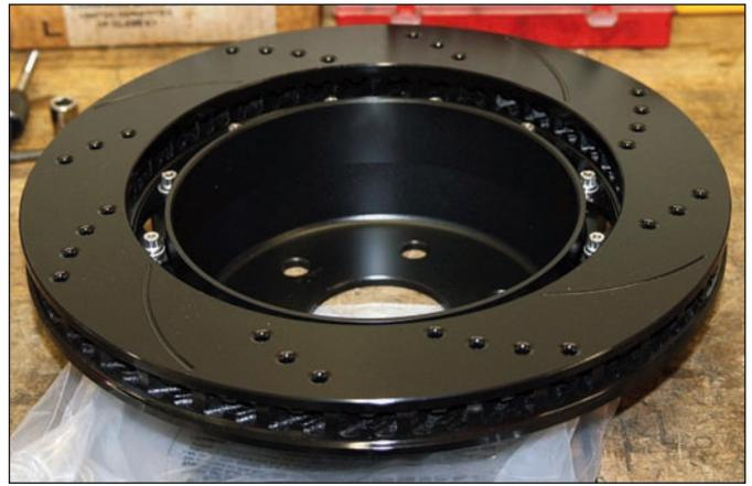
**Sequence 4:** The hat needs to be bolted to the rotor. Orient the rotor over the hat in the configuration shown above. Place one flat washer over each hole on the rotor mounting tabs. Apply red *Loctite*® 271 to the mounting bolts and slide through the washer and thread into the hat.
