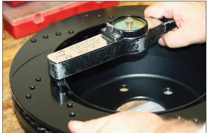
**Sequence 5:** Using an alternating sequence, torque rotor bolts to 140 in-lbs.
