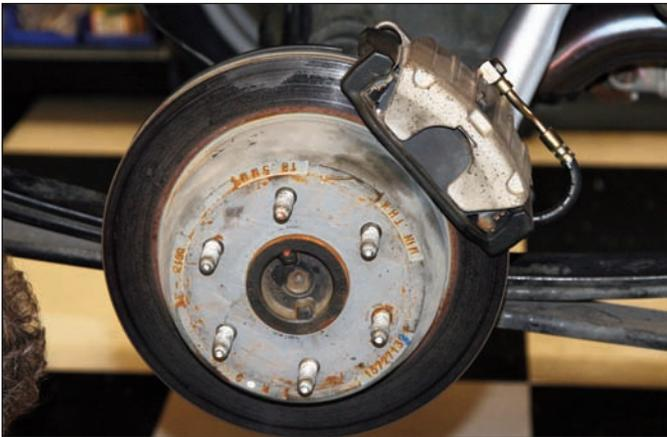
**Sequence 2:** Disconnect the OEM brake fluid hose where it connects to the brake hard line. Temporarily cap (not included) the line to minimize fluid loss. Using an impact driver or breaker bar and socket, break loose the caliper mounting bolts from the back side of the rotor. Lift off the caliper and keep the fluid line hose in the vertical position to avoid spilling brake fluid that remains in the hose.
