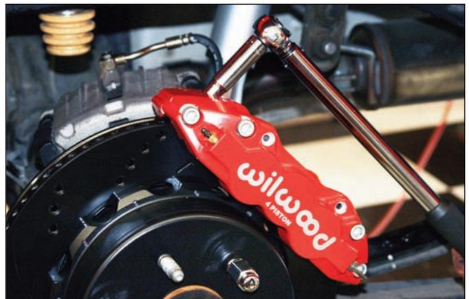
**Sequence 12:** Secure the caliper with washer and locknut, temporarily tighten.
