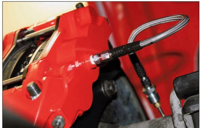
**Sequence 17:** Remove the protective sticker from the caliper fluid inlet. Coat the inlet fitting with PTFE thread tape and screw into the caliper. Connect one end of the Wilwood flexline hose kit, P/N 220-8999 to the fitting. Route flexline along the same path as the OEM hose.
