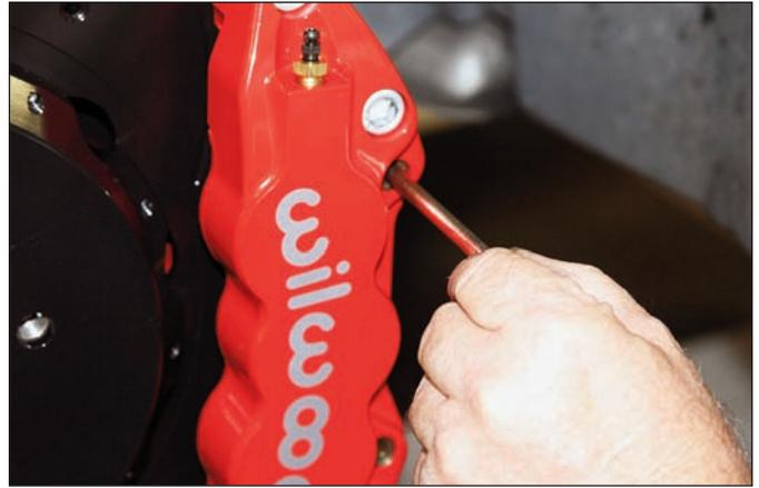
**Sequence 16:** After the pad height is set, install the pad retain pins and secure with the pin retainer clips. Then finalize the caliper mounting by torquing the caliper mounting lock nuts to 47 ft-lb.
