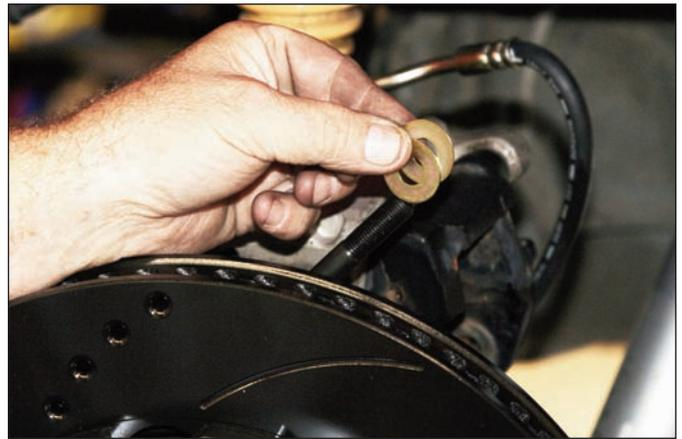
**Sequence 10:** Lubricate the caliper mounting studs with lightweight oil. Initially place two shim washers on each stud between the bracket and caliper.
