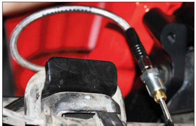
**Sequence 18:** Connect the other end of the flexline to the fitting at the brake hard line. Secure line as necessary to prevent contact with moving suspension, brake, or wheel components. Bleed the system referring to the additional information in the data sheet as necessary for proper bleeding instructions.
