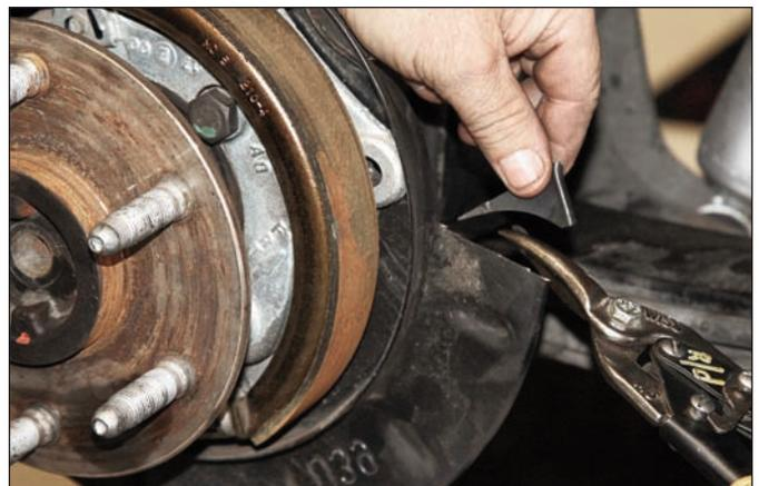
**Sequence 6:** The dust shield needs to be trimmed on both the top and bottom openings for the Wilwood caliper mounting bracket to fit properly. Test fit bracket and trim as necessary. Paint newly exposed areas to prevent corrosion.
