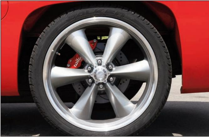
**Sequence 19:** Install the wheel and torque the lug nuts to manufacturer's specification. Rotate the wheel and check for any interference. Bed in the brake pads and rotor in a safe location before general use driving.
