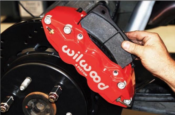
**Sequence 14:** With the pad retain pins removed, insert the brake pads into the caliper with the friction material facing the rotor.
