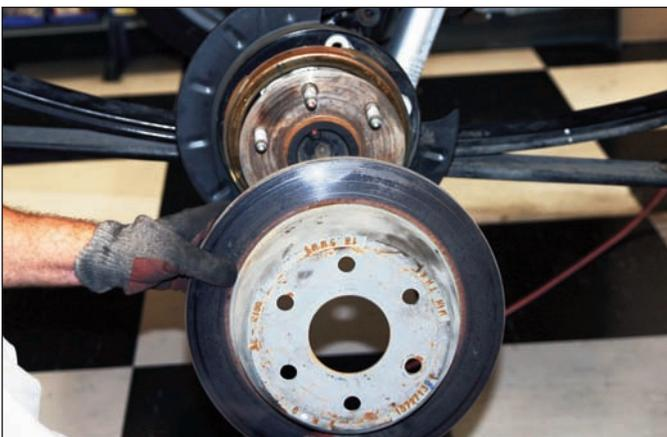
**Sequence 3:** Slide off the rotor from the hub. If it is stuck, it may be necessary to hit it a few times with a rubber mallet to break loose.
