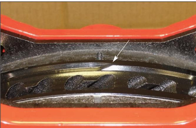
**Sequence 15:** Check that the top of the brake pad is flush with the outside diameter of the rotor (arrow). If not, adjust by adding or subtracting shims between the bracket and the caliper.
