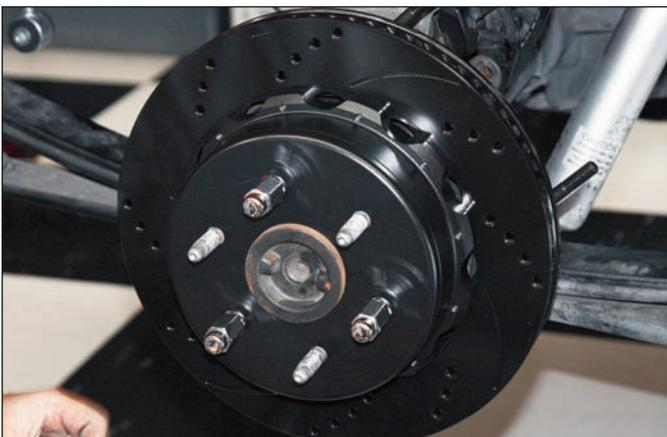
**Sequence 9:** Install the hat/rotor assembly over the hub assembly. **NOTE:** The hat/rotor must fit flush against the axle hub flange or excessive rotor run out may result. Secure the hat/rotor with three lug nuts (finger tight) to keep the hat/rotor assembly in place while continuing with the installation.
